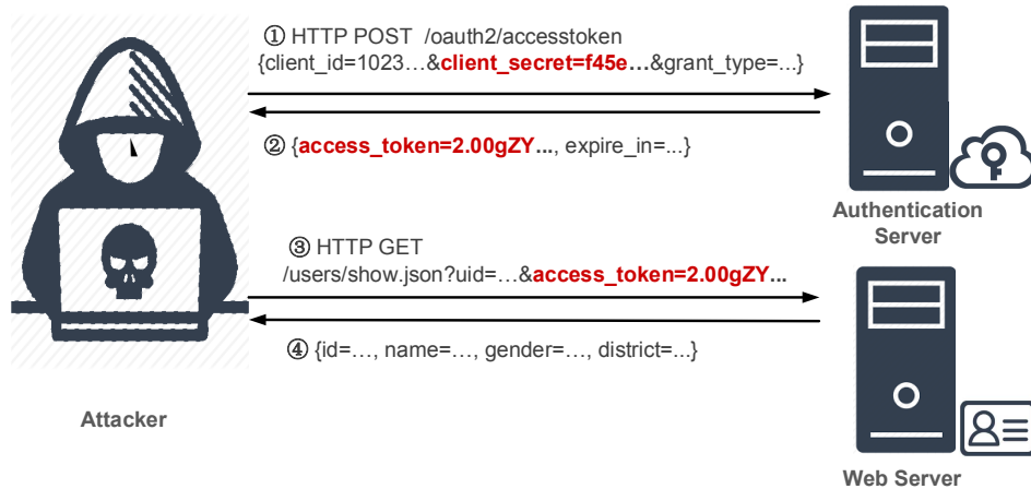
Fig. 2: How can an attacker harvest user information with a valid SDK credential
